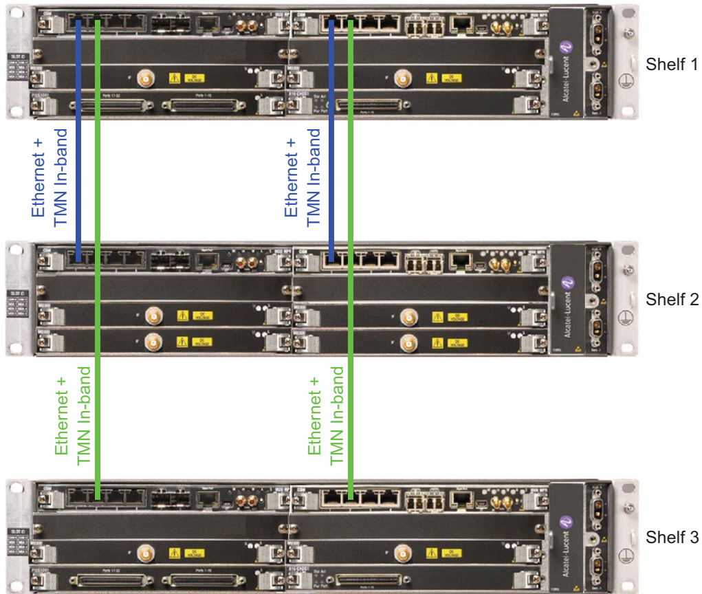
Figure 11. Stacking configuration with 3 MSS with Core protection
