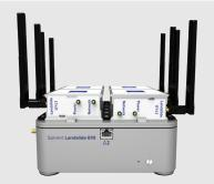
Landslide E10 VTA hosting platform with optional LTE/Wi-Fi over-the-air testing
