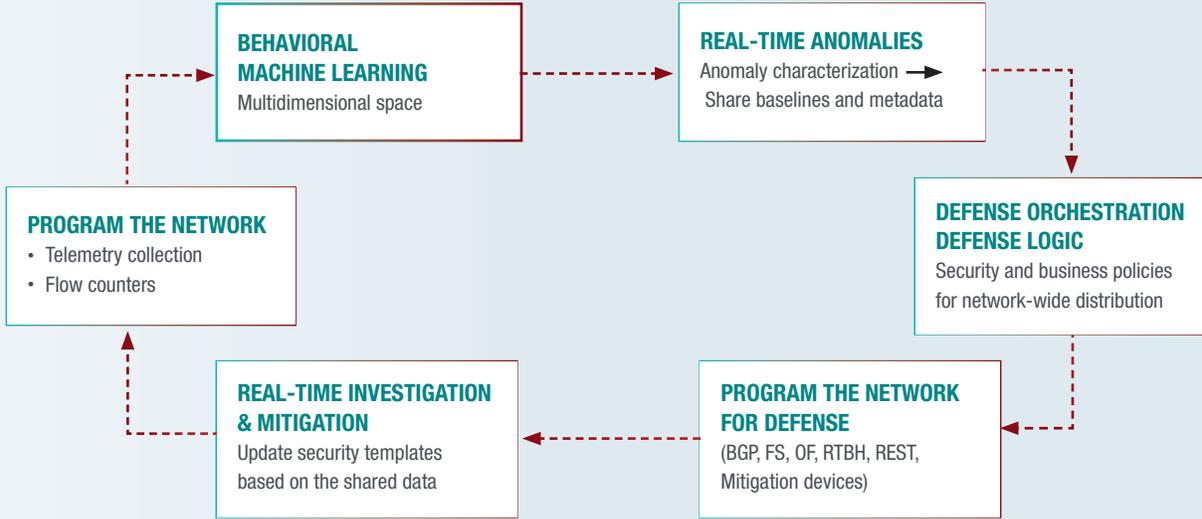
Figure 2: The security automation life cycle
