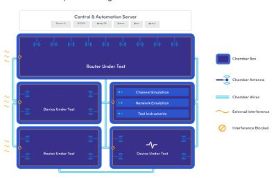
The OCTOBOX STACK provides a modular approach to testing that includes automated testbeds with isolation chambers, antennas, emulators, and test instruments that can be rapidly configured and deployed.
