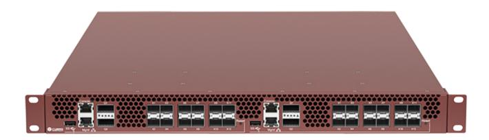
The AGG32100 aggregates, filters and load balances the traffic and forwards the traffic to the session fabric. The session fabric analyzes the traffic and tags it based on application key before forwarding it back to AGG32100. The traffic is sent to other tools for more inspection.
