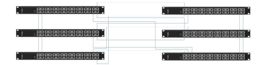
In this application 6 x AGG32100s are connected to a fully meshed cross connect with 162 available 100 Gbps ports (27 available ports per device). The interconnection between the devices can be done with one link or more depending on the bandwidth that is needed.
