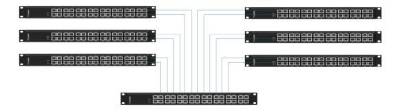
In this application 6 x AGG32100s are connected to a central unit with 186 available 100 Gbps ports (31 available ports per device).
