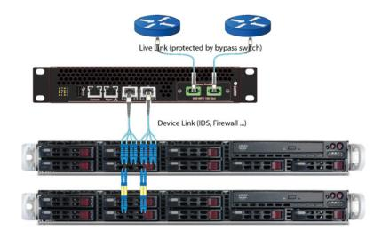
The output for the inline device load balanced is 4 x 25 Gbit or 4 x 10 Gbit.
