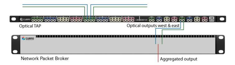
By utilizing the various filtering capabilities of the EXA48200 the user is able to further reduce traffic volume that needs to be processed, thus enabling quicker and more accurate analysis and troubleshooting. Moreover, incoming traffic can be VLAN tagged per physical port to allow easy identification at which physical port a packet original arrived.
