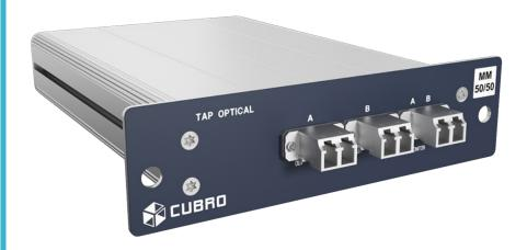
An optical TAP gives you real-time monitoring access to a physical optical data link without interfering it. Due to the fact that the optical TAP is fully passive (no power supply needed) it is no risk to put it in an active link.
