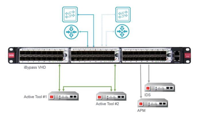
iBypass VHD flexibility example: with a failover network connection configured, iBypass VHD passes the traffic from a single network link to two serial inline tools and creates copies of the same traffic that is regenerated to two additional out-of-band tools.
