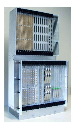
The SMA16-64 is the family of new-generation, full-feature, compact Add-Drop Multiplexer (ADM) and Digital Cross-Connect (DXC) with full, non-blocking, VC-12 cross-connection capability.
