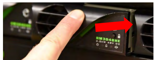
Figure 14: Inserting a Rectifier
